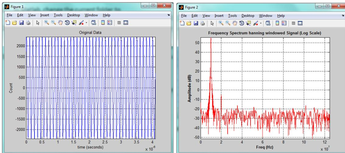
In the figures above, we clearly see the 10MHz tone in the time spectrum plot and the frequency spectrum FFT plot.
